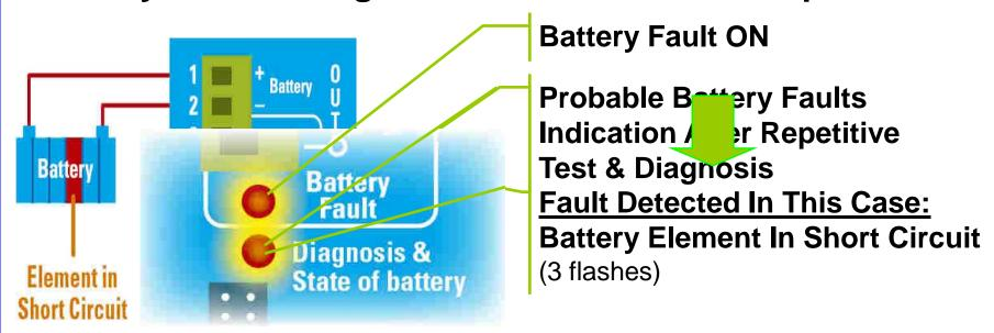
With a pulse sent to the battery by a specific circuitry and by evaluating algorithmically the received signal, it is possible to discriminate battery faults such as cells in short circuit, wire disconnection, etc....
