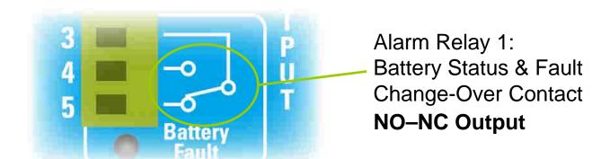
Alarm Relay 1 Battery Low or
