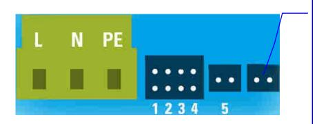
Via RTCONN remote connections cable it is possible to drive the devices from Boost to Trickle charge
