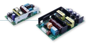
**Output:** Triple output power supply without minimum load requirement
