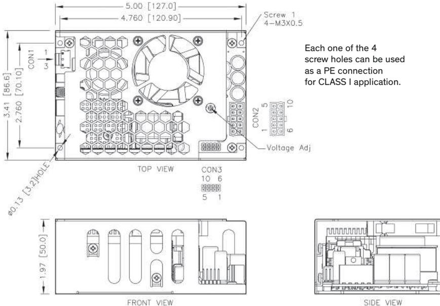
Each one of the 4 screw holes can be used as a PE connection for CLASS I application.
