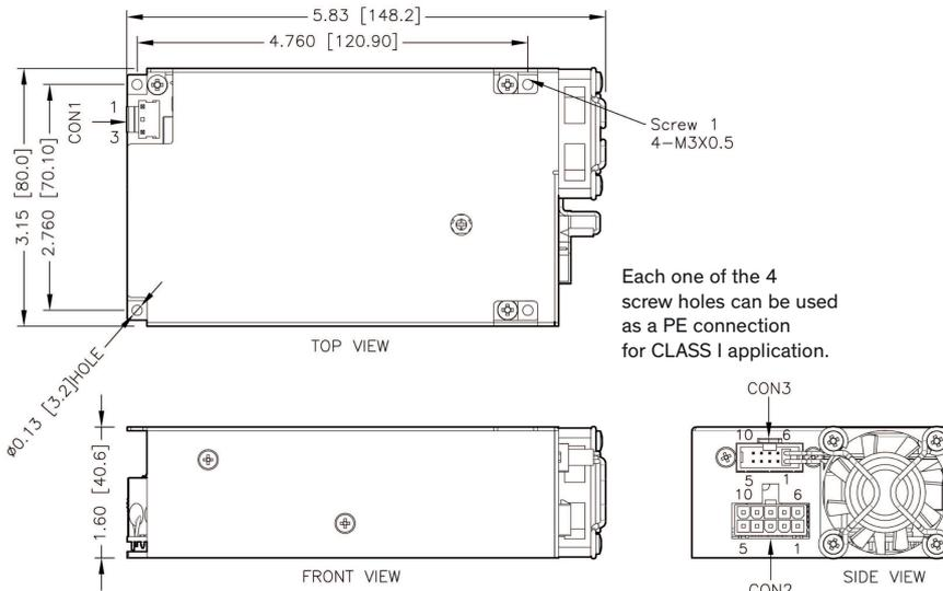
Each one of the 4 screw holes can be used as a PE connection for CLASS I application.
